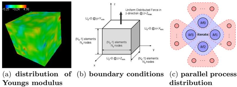
**Fig. 1.** Simple cube geometries with heterogeneity as domains for 3D linear elasticity problems and parallel approach
